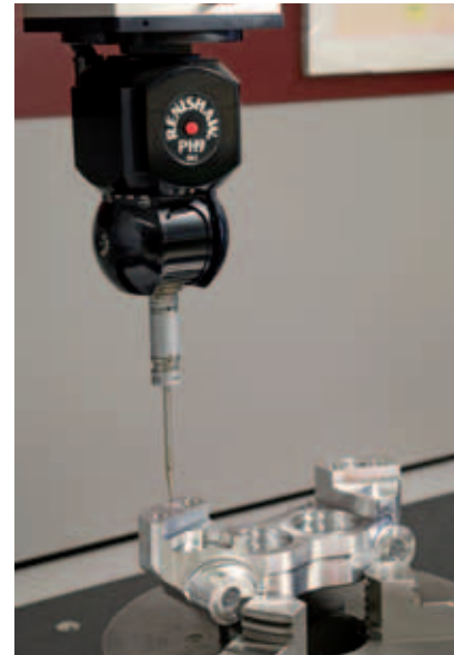
The racing plant in Curno. Checks of the first caliper workmanship phase with a three-dimensional machine.
