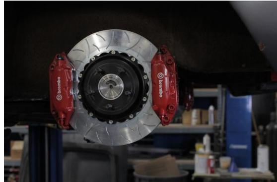
Brembo engineered a unique braking system which consisted of a custom dual circuit configuration for the rear with two pair of 4-piston aluminum alloy calipers. One pair is used for conventional braking, while the other is connected to a hydraulic handbrake for vehicle dynamic control that establishes drifting; something the movie is well known for.
